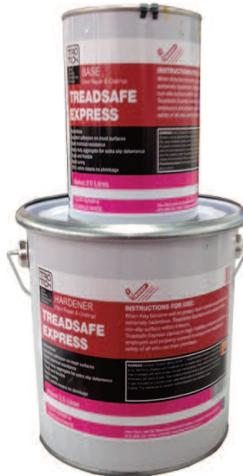
Ensure that the area to be coated is sound and free from oil, grease and loose material. If necessary, prepare the concrete with Concrete Etch. Non porous surfaces may be cleaned and degreased using Multi Clean. Any form of vegetation or mould may be removed by using Multi Wash. The substrate temperature should be between 10°C to 30°C for the application. Mechanically abrade the area to provide a key for the coating.
